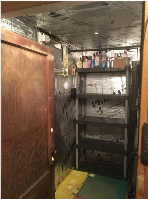
A room in the basement was converted into a walk-in cool room using a CoolBot controller, rigid insulation, and a window A/C unit.
